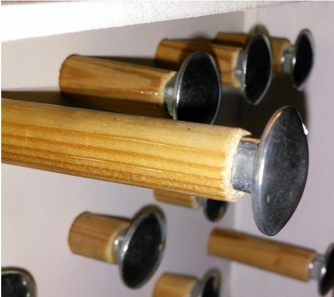
J.2; Image showing our final idea for the pins, with the half spheres at the end.
